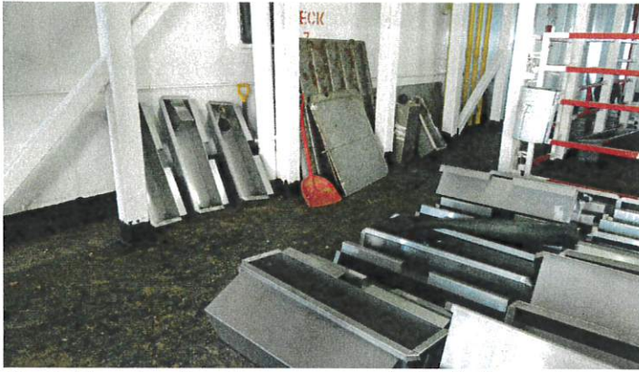
Fig 9. New feed and water troughs built by technicians on-board during voyage 115
